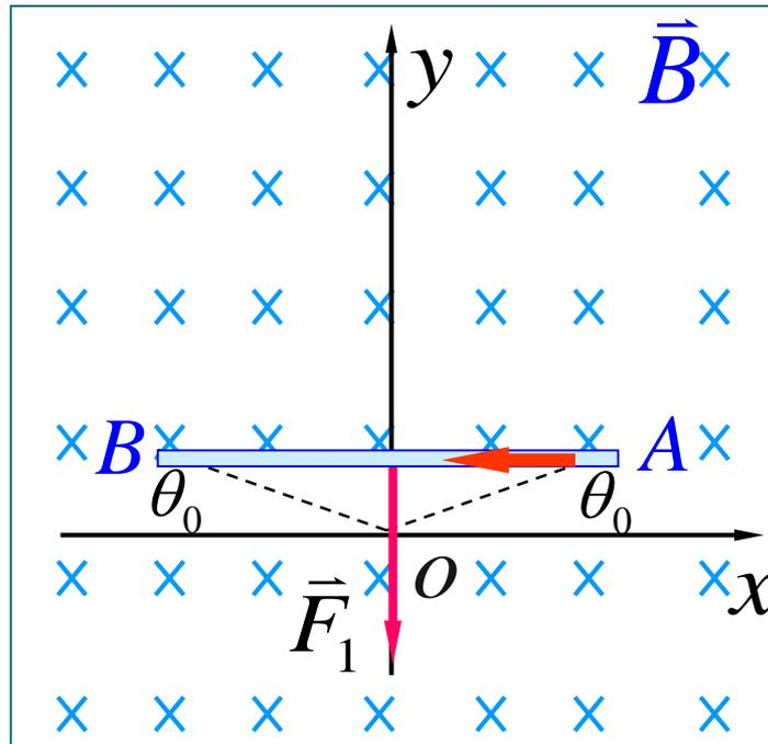
$$\begin{aligned} F_1 &= I \overline{AB} B \\ &= IB 2r \cos \theta_0 \end{aligned}$$
